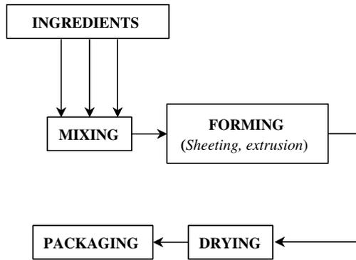
Fig. 1. Pasta production process flow sheet.
